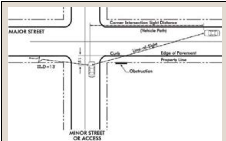
Figure 4-17: Corner Sight Distance (no on-street parking)
