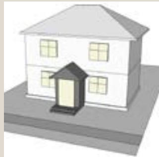
Portico with Peak Roof
