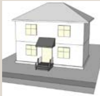
Stoop with Shed Roof
