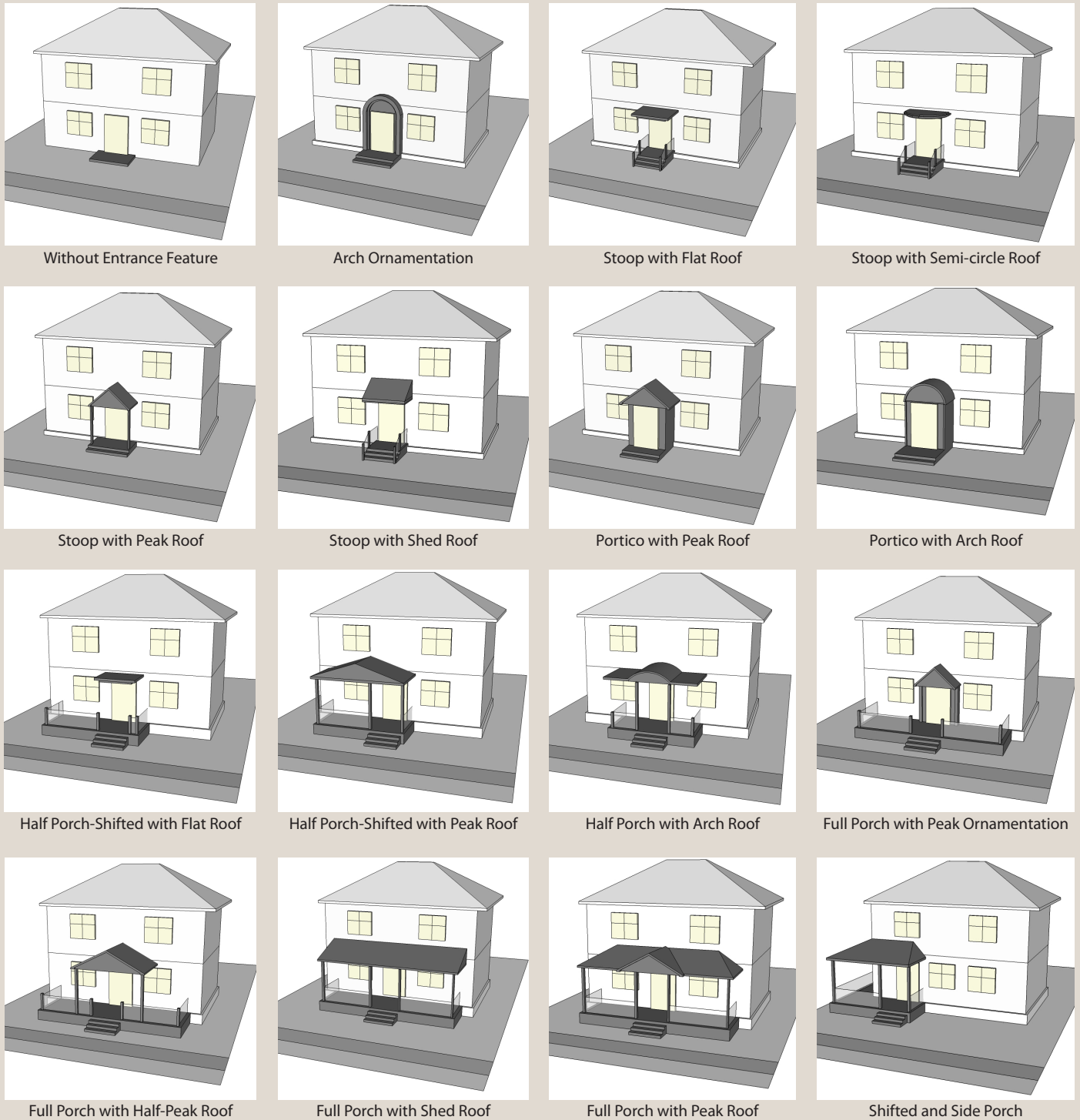
Figure 6-9: Residential Building Entrances
