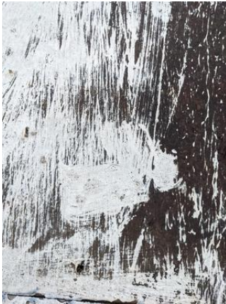
CHE-SP7078-180821-004 thru 006, Asbestos Not Detected, White sealant
