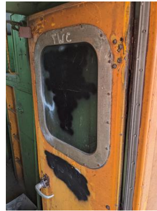
CHE-DRGW01489-150721-001P, PCB Not Detected, Black window caulk
