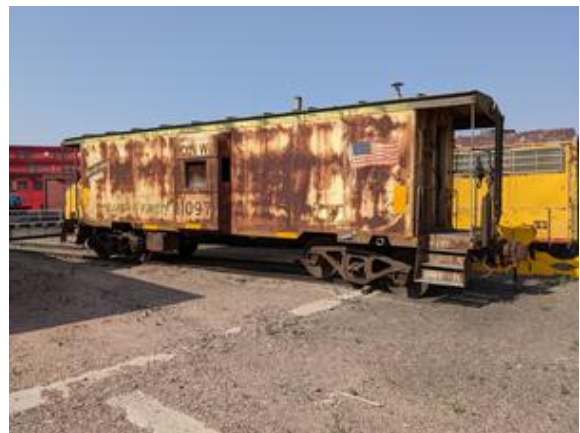
CHE-CNW11097-140721-002L, 0.014% Lead, Yellow
