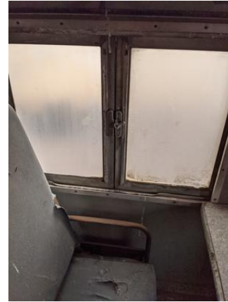
CHE-MP13835-130721-010 thru 012, Asbestos Not Detected, Gray window glazing
