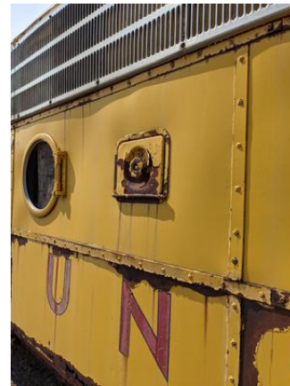
CHE-UP928-160821-013 thru 015, Asbestos Not Detected, Yellow/Black Penetration Gaskets
