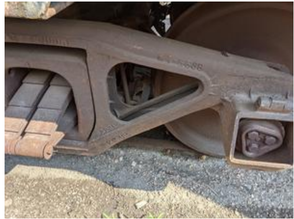
CHE-CNW11047-150721-010 thru 012, Asbestos Not Detected, Black brake pads
