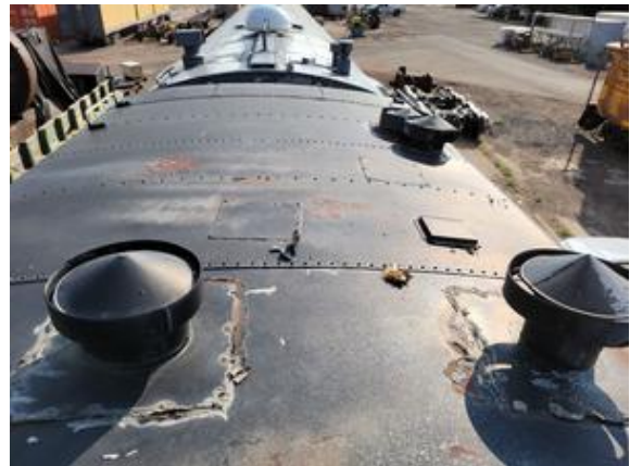
CHE-SP7077-170821-001P, PCB Not Detected, Clear silicone caulk
