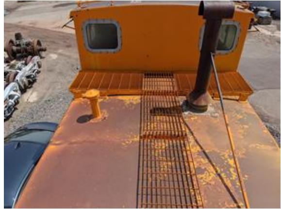
CHE-DRGW01489-150721-010 thru 012, Asbestos Not Detected, Black tar
