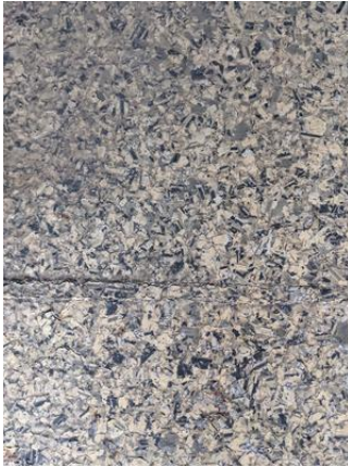
CHE-MP13835-130721-001 thru 003, Asbestos Not Detected, Beige flooring and beige mastic
