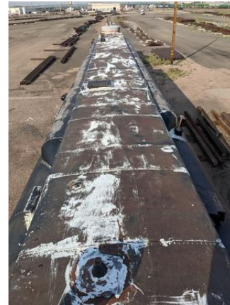
CHE-SP7078-180821-004 thru 006, Asbestos Not Detected, White sealant
