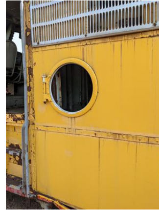
CHE-UP928-160821-019 thru 021, Asbestos Not Detected, Black window gasket
