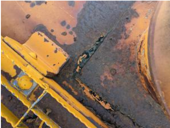
CHE-DRGW01476-170721-013 thru 015, 6% Asbestos, Black tar
