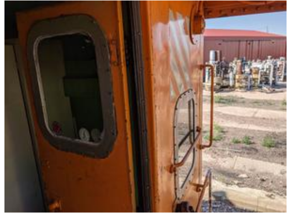
CHE-DRGW01476-170721-001P, PCB Not Detected, Gray/black window caulk
