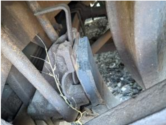
CHE-CNW11111-150721-013 thru 015, Asbestos Not Detected, Black brake pads
