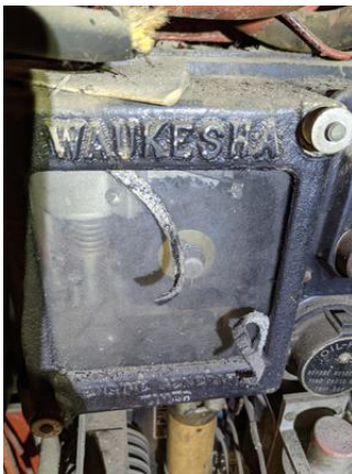
CHE-SP7078-180821-031 thru 033, Asbestos Not Detected, Gasket (layered silver coating and black felt)
