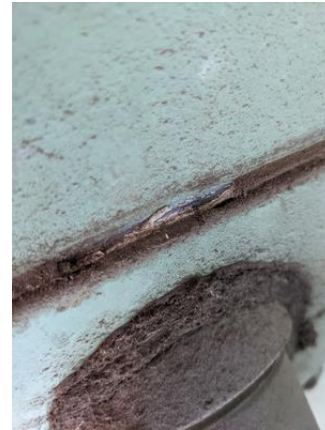
CHE-SP4641-130721-022 thru 024, 10% Asbestos, Gray oil tank sealant
