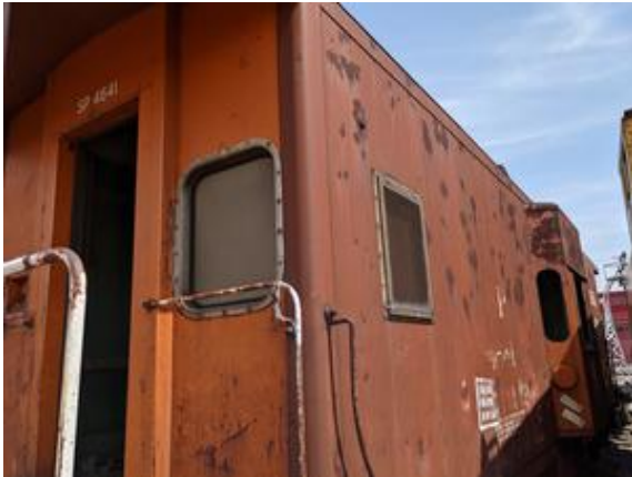
CHE-SP4641-130721-002P, PCB Not Detected, White window caulk
