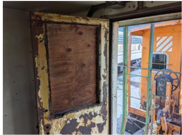
CHE-CNW11111-150721-010 thru 012, Asbestos Not Detected, Gray caulk
