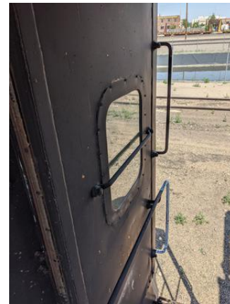
CHE-DRGW01486-160721-001P, PCB Not Detected, Black window caulk
