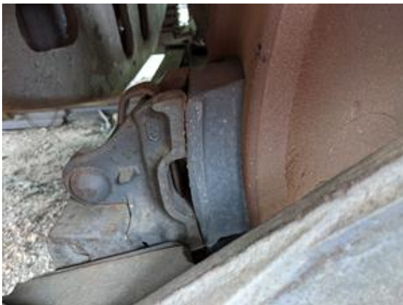
CHE-FTSX812-140721-016 thru 018, Asbestos Not Detected, Black break pads
