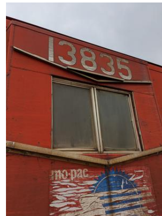
CHE-MP13835-130721-025 thru 027, 10% Asbestos, Gray window caulk
