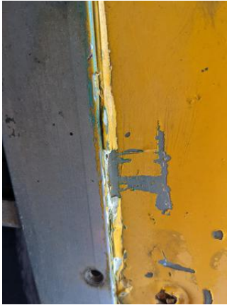
CHE-FTSX812-140721-010 thru 012, Asbestos Not Detected, White sealant
