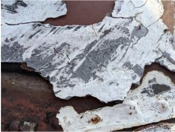
CHE-SP7078-180821-001 thru 003, 8% Asbestos, Black/gray sealant
