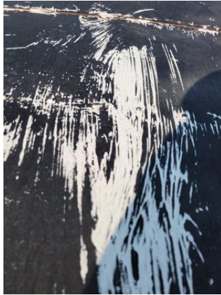
CHE-SP7077-170821-007 thru 009, Asbestos Not Detected, White sealant
