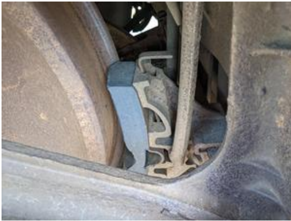
CHE-CN11097-140721-010 thru 012, Asbestos Not Detected, Black brake pads
