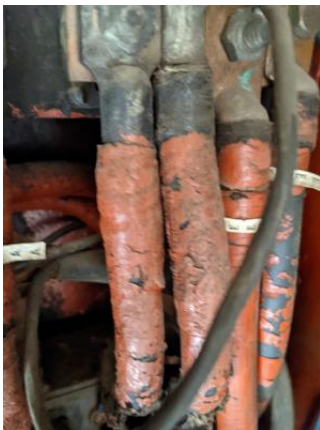
CHE-SP7078-180821-022 thru 024, Asbestos Not Detected, Red/Black wire coatings
