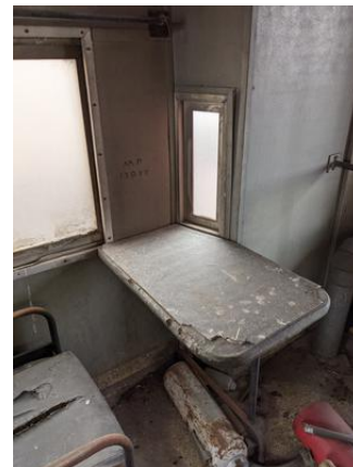
CHE-MP13835-130721-007 thru 009, Asbestos Not Detected, Linoleum table top (no mastic)
