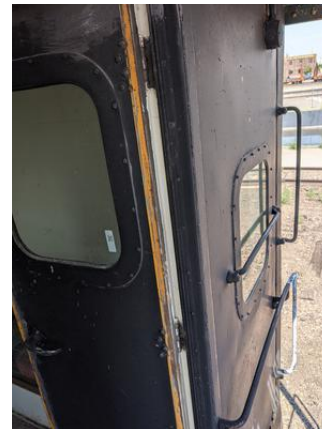
CHE-DRGW01481-160721-001P, PCB Not Detected, Black/brown window caulk
